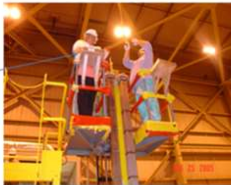
ANSI N.45.6, LEVEL III OGLE, PERFORMING NEW FUEL BUNDLE RECEIPT INSPECTION WHILE BUNDLE IS SEATED, IN INSPECTION STAND, AFTER THE UPPER TIE PLATE WAS REPLACED BY G.E.
