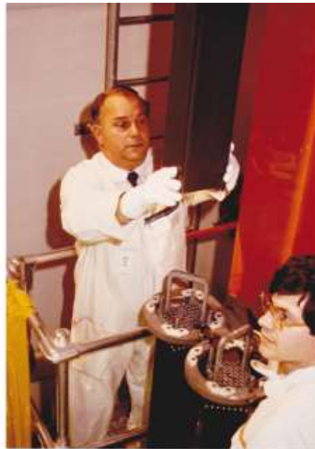
Charlie Ogle Level III at KKL Site. Training KKL Fuel Inspector on how to channel a New Fuel Bundle.
